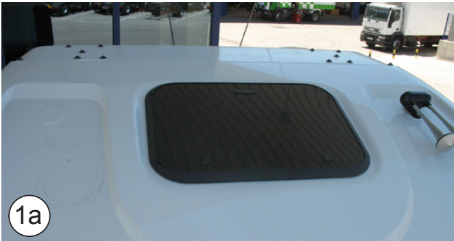
Stralis Cabin before 2008: 40 x 40 EPDM joint
